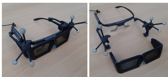
Figure 3: An assembly combining a system of Vulfoni stereoscopic glasses with Tobii 2 eye tracking glasses, attached together with a 3D-printed clip which is also designed as the tracking constellation system.
