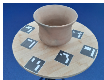
Figure 4: Augmented Reality markers (ArUco fiducial markers) placed around the object of interest in order to track the participants' position relative to the object.
