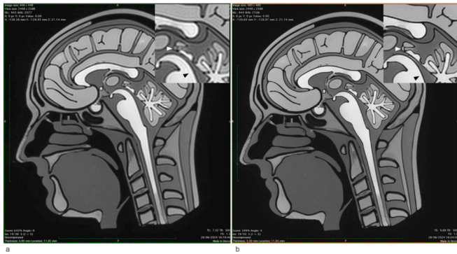
Fig. 4. Image quality comparison between acquisition 1 (a) and acquisition 4 (b) (see Table 3). We can see that truncation artefacts (black arrowhead) are more pronounced on acquisition 1 (a), while anatomical details are more visible (white arrowhead) on acquisition 4 (b). This is linked to the increase in the size of the acquisition matrix (see Table 3). The use of these phantoms therefore looks interesting both for qualitative analysis of sequences and for training in normal anatomy.
