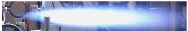
FIG. 1. Low acquisition-rate and slow shutter speed imaging of the afterburning, as recorded by a regular camcorder (multimedia available online).
