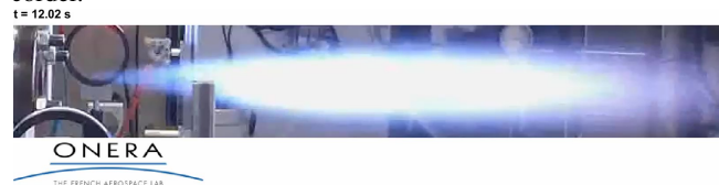
FIG. 27. Supplementary Material S1: Low frame-rate, slow shutter speed imaging of the afterburning recorded by a regular camcorder.
