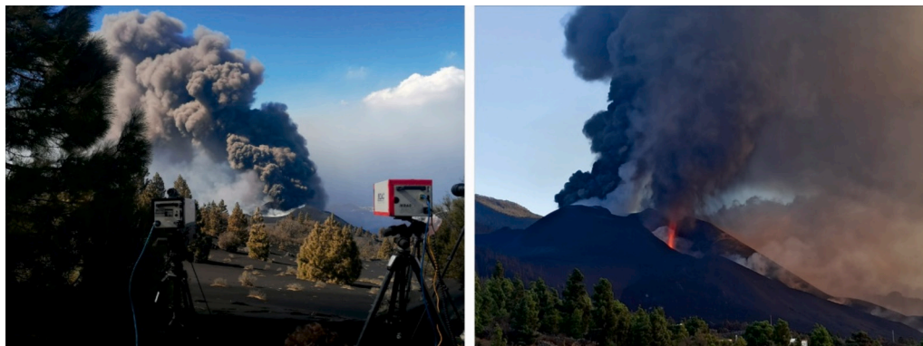
Fig. 4. (A) Picture taken November 8, 2021, showing the two FTIR spectrometers operated simultaneously. A very ashy plume can be observed. (B) Picture taken October 28, 2021, where the plumes overlapped with W-E wind.
