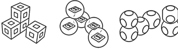
Fig. 17. a) MRB reconfiguration using magnets. b) MSRR self-reconfiguration using CPU and I/O. c) MSRMR Morphing self-reconfiguration using actuators.
