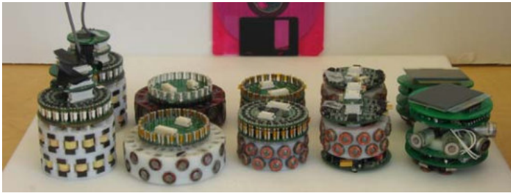
310 311 312 313 314 315 316 317 318 319 320 Fig. 3. Different prototypes of planar catoms (V2 to V6) [retrieved from: http://www.cs.cmu.edu/~claytronics/hardware/planar-stuff/catomelectromagneticmodules.pdf ] 321 322
