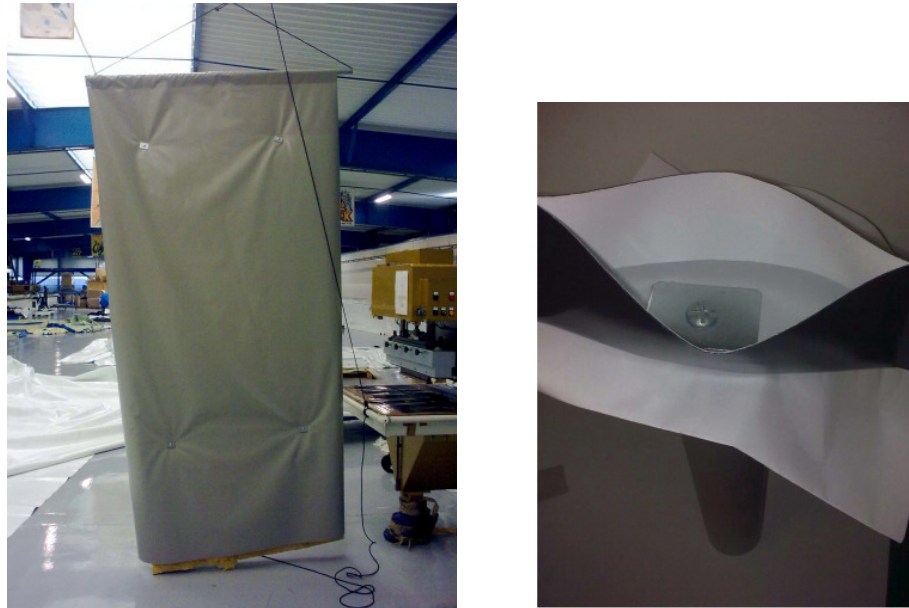
Figure 11 : Tensile insulation support : large prototype and water tightness testing of the bolts
