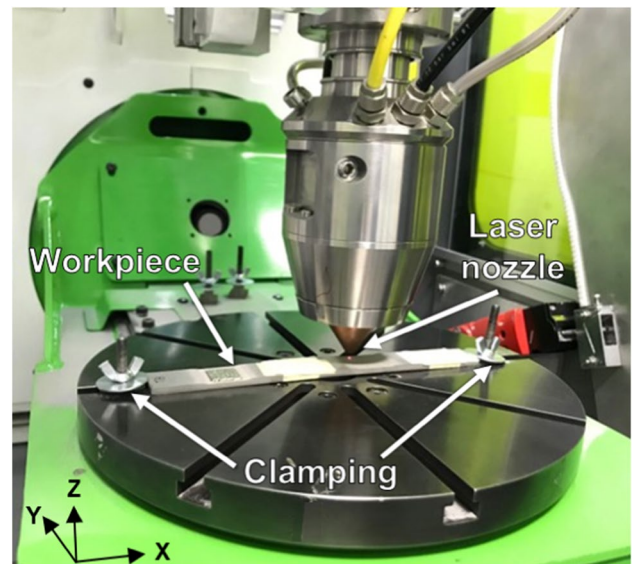
Fig. 2 Overall view of the experimental setup for Laser Metal Deposition process
