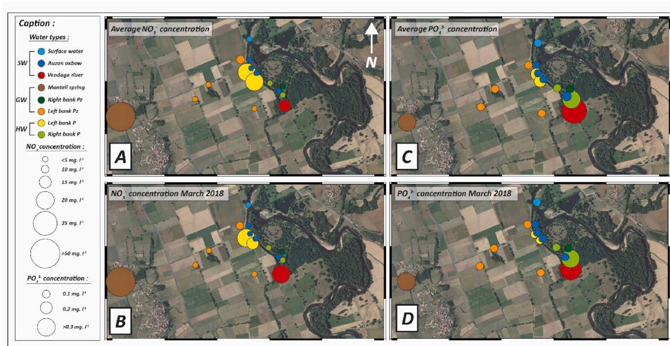
Fig. 2. Nitrate and phosphate concentration maps based on the concentrations recorded during the 44 sampling campaigns on the Auzon oxbow. (A) Mean \text{NO}_3^- concentrations during the 2014–2018 period; (B) \text{NO}_3^- concentration during the March 2018 campaign; (C) Mean \text{PO}_4^{3-} concentrations during the 2014–2018 period; (D) \text{PO}_4^{3-} concentration during the March 2018 campaign.
