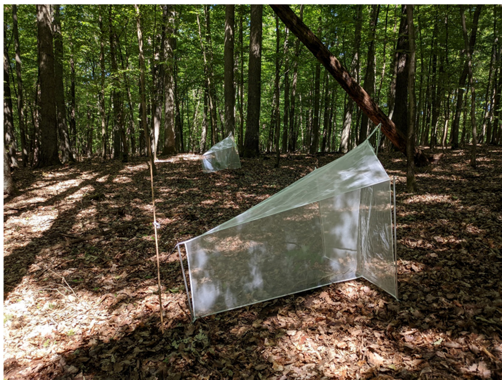
Figure 1. A pair of Malaise traps placed over oak saplings in Puszcza Zielonka forest, Poland. The sapling is situated behind the central screen.
