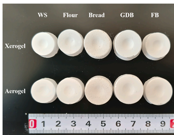
Fig. 3. Morphology of xerogels and aerogels made from wheat starch (WS), wheat flour (Flour), bread particles (Bread), gluten-depleted bread particles (GDB) and finely milled bread particles (FB).
