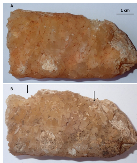
Figure 4. Evolution of a speleothem from Orgnac Cave after 55 days in guano suspension at 80°C, A: before experiment, B: after immersion in guano suspension. Sparite crystals have been dissociated by intercrystalline dissolution. The arrows indicate areas where the sparite crystals broke up during scraping.
