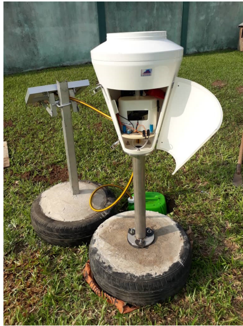
Figure 2. A Precis Mécanique ® tipping bucket rain gauge equipped with a remote transmission system. The top of the rain gauge is 1.5 m above the ground, in accordance with WMO standards. The green can, buried between the two tires, is the totalizer used to check that the tilts correspond to the amount of rain collected. The mast on the left carries the solar panel used to recharge the battery of the remote transmission system. The rain gauge reference from Precis Mécanique ® is model 3039 resolution 0.5 mm (untouchable, extended range 0–1000 mm/h). Patented mechanical system 1154024/400 cm 2 cone.
