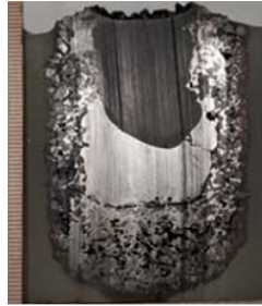
Figure 10: Cross section obtained after progression of molten steel through a debris bed (CORDEB CD5-03) test [39].
