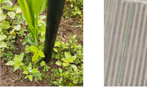
Fig. 5: (left) RTK GNSS antenna position when recording crops positions – (right) recorded RTK GNSS paths
