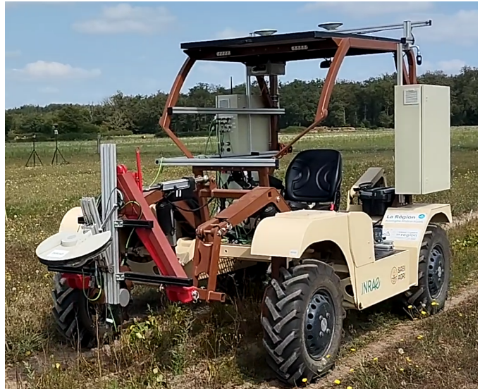
Fig. 1: POM4x4 of Sabi Agri manufacturer, here configured with a 2D lidar at the front
