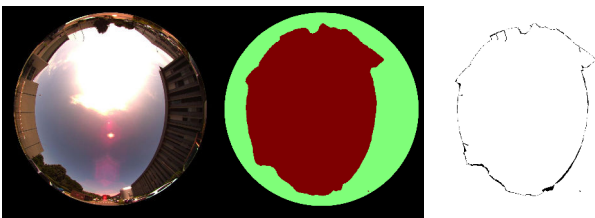
Fig. 3. Example of segmentation error compared to the ground truth labelled by an expert : (left) original image; (middle) predicted segmentation; (right) segmentation error.
