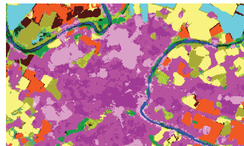
(d) Pixel and edge density features, in a sliding window of size 11 \times 11 . Some corners are preserved, but some are rounded.
