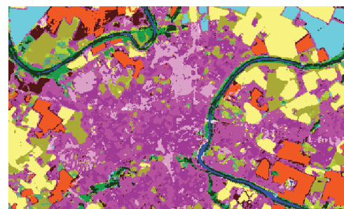
(b) Baseline: Pixel-based classification by Random Forest. The main sources of errors are noise, and the lack of context.
