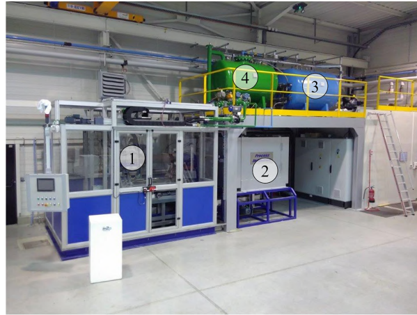
Figure 1: Photograph of the large-scale cooling experimental bench: 1) cooling chamber; 2) furnace; 3) compressed air tank; 4) pre-heated water tank. [19]
