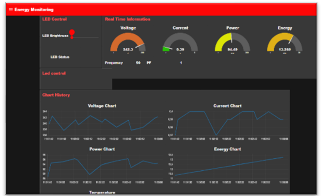
Fig. 4. Electric parameters Dashboard interface
