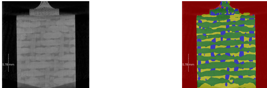
(a) A tomographic slice of a woven carbon fiber reinforced polymer sample.
