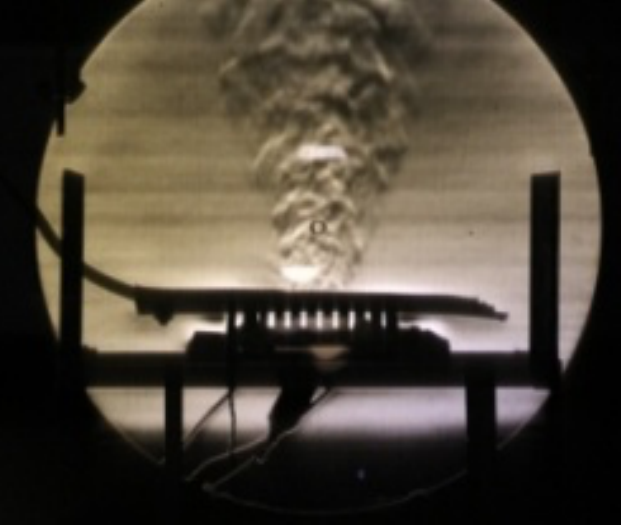
Fig. 2. Schlieren optics visualization of forced ionic wind convection powered under 7 kV.
