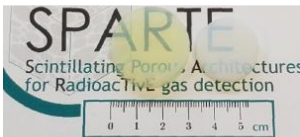
Fig. 1 - Aerogels before (left, \text{Ce}^{3+}:\text{YAG} , yellow sample) and after (right, \text{Ce}^{4+}:\text{YAG} , white sample) thermal treatment
