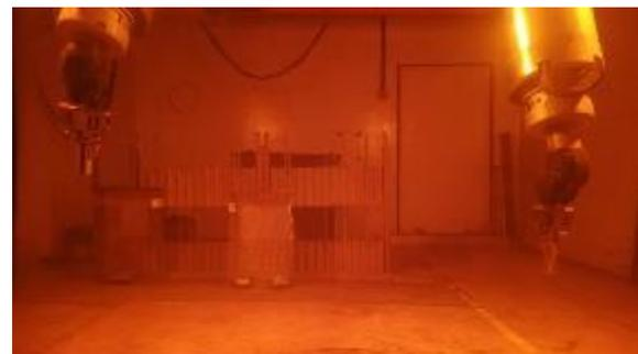
FIG. 2.2. Set-up in the irradiation chamber of batches of masks before gamma irradiation in ARC-Nucléart irradiator
