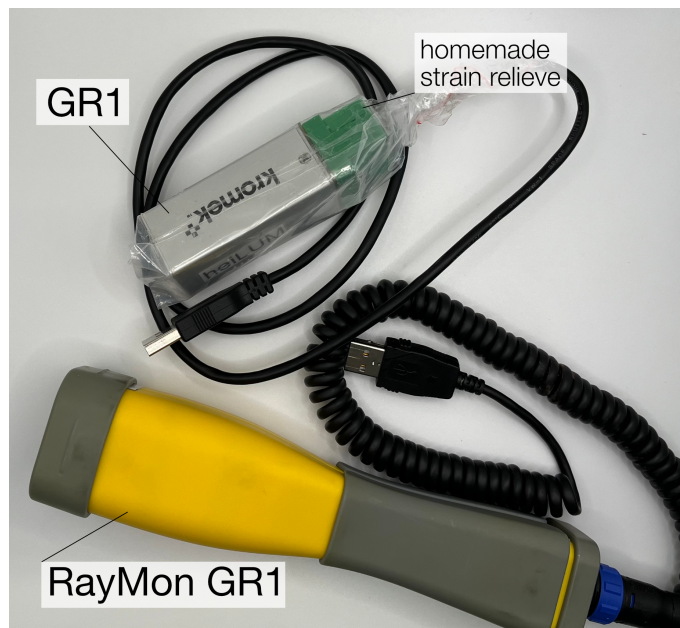
Figure 1. Kromek detectors used for our measurements (shown is the probe without the handheld tablet PC for the RayMon10 ® ). Both probes house a similar CZT detector. We wrapped the GR1 ® in a standard plastic bag and attached a home made strain-relieve to the GR1 ® to enable easier operation and retraction of the detector in the field.
