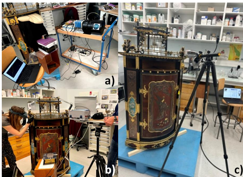
Fig. 2. Examples of instrument positioning: a) remote Raman head connected to the laser and spectrometer (black cylinder) by optical fiber; note the black fabric protecting the eyes against scattered laser light and the spectra against pollution of the measurement by lighting; the sheets of paper adjust the height of the spot and eliminate vibrations; b) FTIR spectrometer on its micrometric displacement support; c) in-situ XRF setup.
