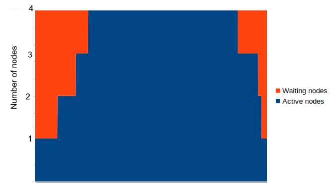
Figure 3: The number of nodes used to execute our workflow of 4 Pods using the autoscaling mechanism in infrastructure_1
