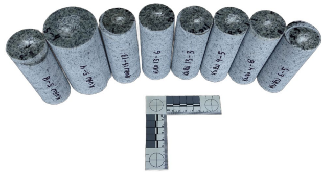
Fig. 12 Core samples of Kuru granite scanned by XCT
