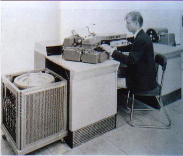
Figure 2. A picture of the CAB 500 computer (designed by the French company SEA, around 1957, by Alice Recoque. [Starynkevitch 1990])
