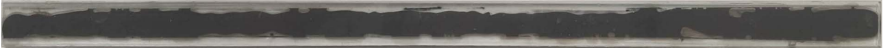
Figure 10. Sample G1 , a glass beam with a varying quality of the coupling.
