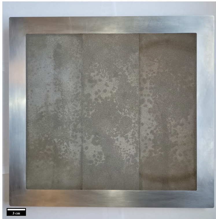
Fig. 4 SPS panels assembled on its frame
