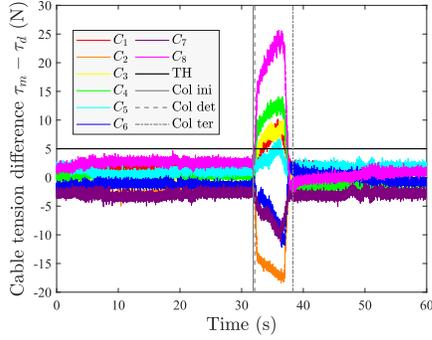
Fig. 4. Difference between measured and desired cable tensions during a collision event from 31.873 s to 38.317 s. Here,  $C_j$  denotes the  $j^{th}$  cable of the CDPR,  $j = 1, 2, \dots, 8$ ; 'TH' represents threshold  $T_h$ ; 'Col' stands for collision; 'ini' for initialization; 'det' for detection; and 'ter' for termination.
