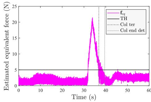
Fig. 12. Equivalent force  $f_{eq}$  with the collision management strategy for cable 8, referring to collision case in Fig. 11, where the collision ends around 36.980 seconds and is detected at 39.503 seconds.
