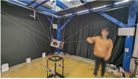
Fig. 3. Collision test between a human operator and a cable on the CRAFT platform<sup>2</sup>.
