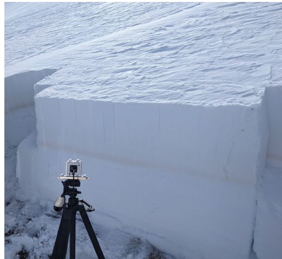
Figure 2: Event sensor placed in front of the snow beam during session 2.
