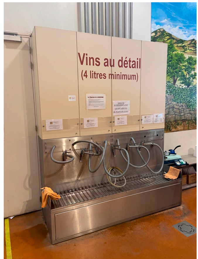
Fig. 4. Cooperative equipment for dispensing wine into re-useable bidons, a marker of the productivist era in that wine is dispensed in bulk, but perhaps also prefiguring more sustainable forms of local wine distribution.?. NOTE: This photo is not from the cooperative at which Y worked. Photo by one of the authors.
