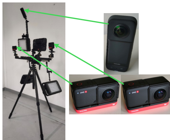
Figure 1. The SQUILLIDAE set-up mounted with a 360° cameras triplet
