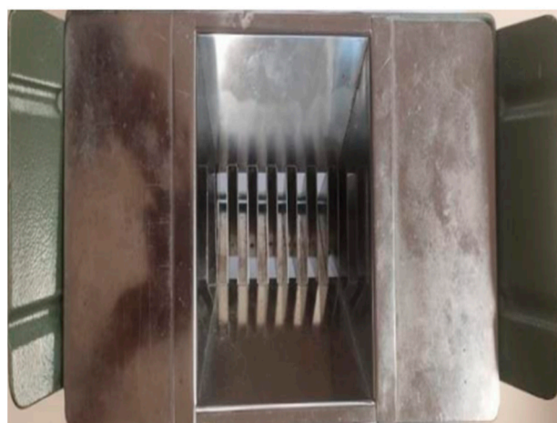
Figure 4. The material divider for sampling the products of the electrostatic separation experiments.
