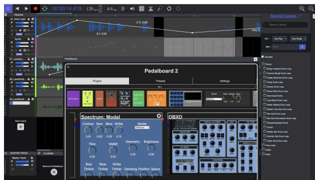
Figure 1: WAM Studio typical view, showing audio and MIDI tracks with some parameter automation curves and the plugin chain associated with the selected track.
