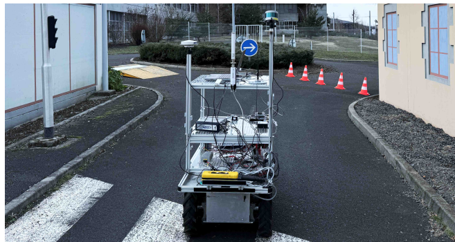
Fig. 1. An illustration of a scenario where a robot must successfully navigate through a speed bump to reach a position behind the roundabout. Using our framework, the vehicle is able to cross this environment while considering the risks involved during navigation.
