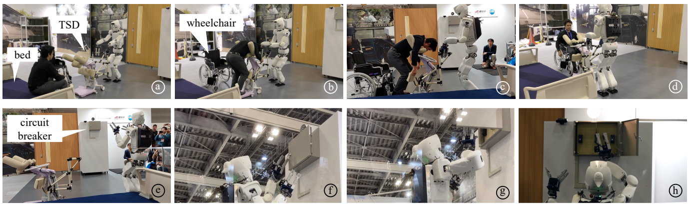
Fig. 10. Demonstration scenarios at IREX. ① The bed is tracked, and the TSD is taken in front of the patient. ② The TSD is operated wirelessly to support/lift the patient. ③ Turning the TSD with the patient on board toward the wheelchair. ④ The TSD is operated wirelessly, and the patient is lowered to sit in the wheelchair. Then, the patient asks to investigate a problem with the light. ⑤ The robot switches to teleoperation mode and moves to the front of the circuit breaker. ⑥ The robot opens the breaker box by turning the door handle. ⑦ The robot hooks the gripper on the lever and opens the breaker box door. ⑧ The robot operates the corresponding breaker switch to turn on the light.
