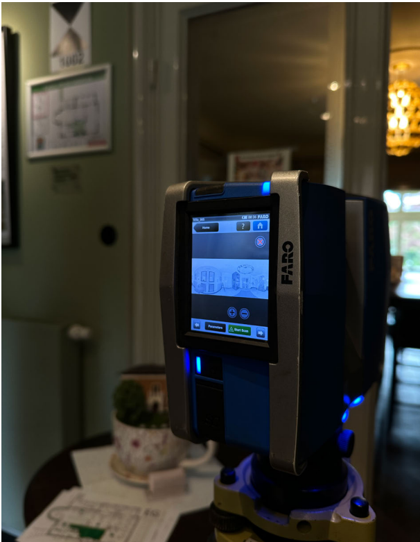
Fig. 2.1.9: Touch screen with scan of the corridor-ground floor
