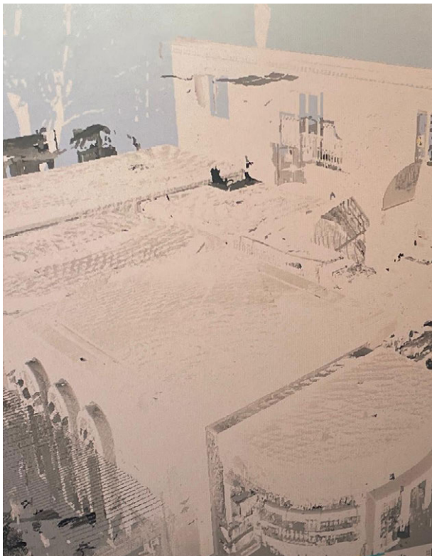
Fig. 2.1.14: First generated point cloud with all scans
