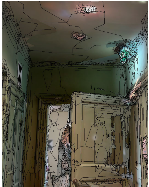
Fig. 2.6.35: Screenshot Archicad, two overlapping scans
