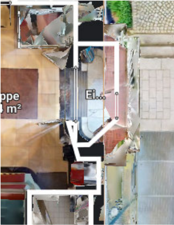
Fig. 2.2.16: Autom. generated floor plan with corner instead of rounding
