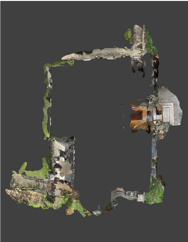
Fig. 2.6.16: Screenshot Scaniverse, incorrect angles of the exterior walls
