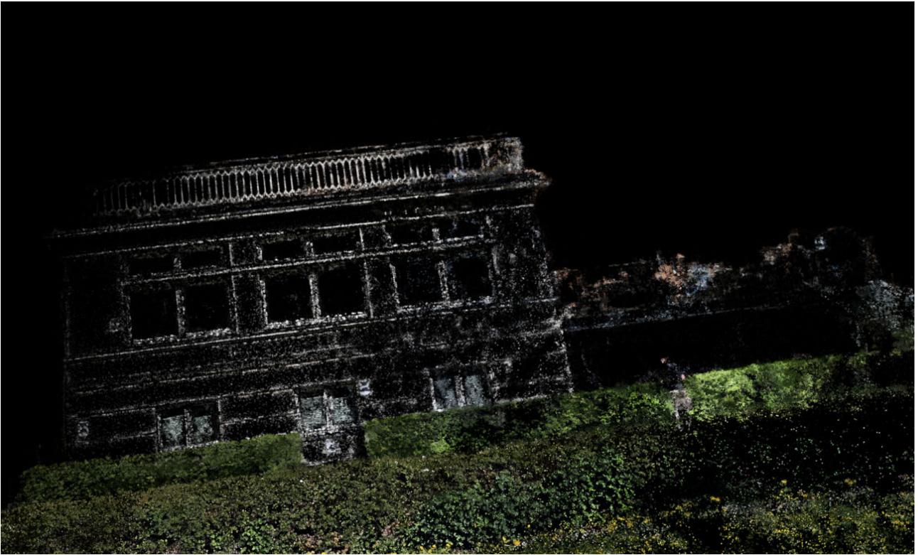
Fig. 1.1.7: Point cloud using NERF technology
