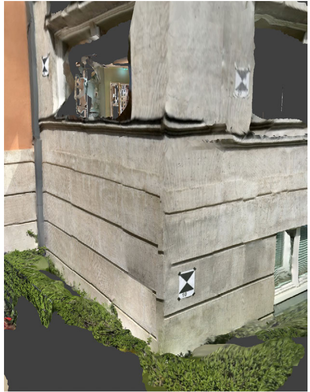
Fig. 2.6.15: Screenshot Scaniverse, misalignment of the heights
