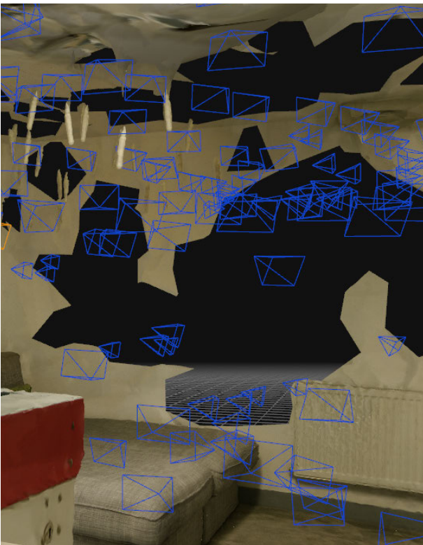
Fig. 2.4.21: Photogrammetry Results of the Basement from 3DF Zephyr
