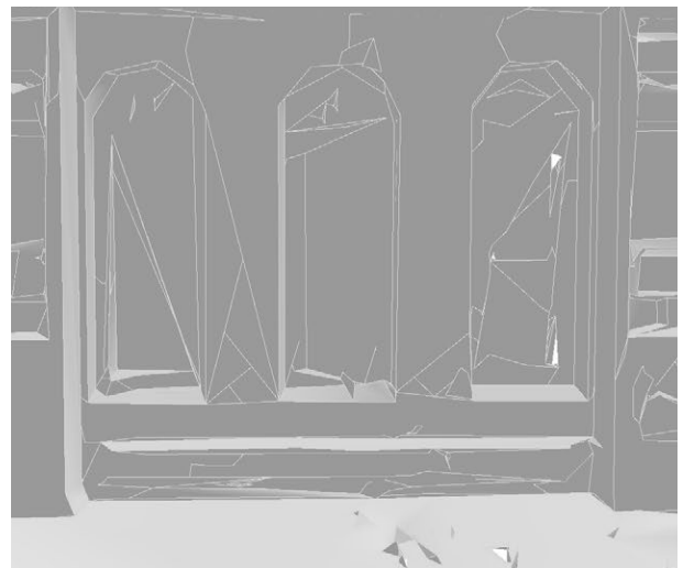
Fig. 2.2.33: Missing window sills of the .3dm mesh
