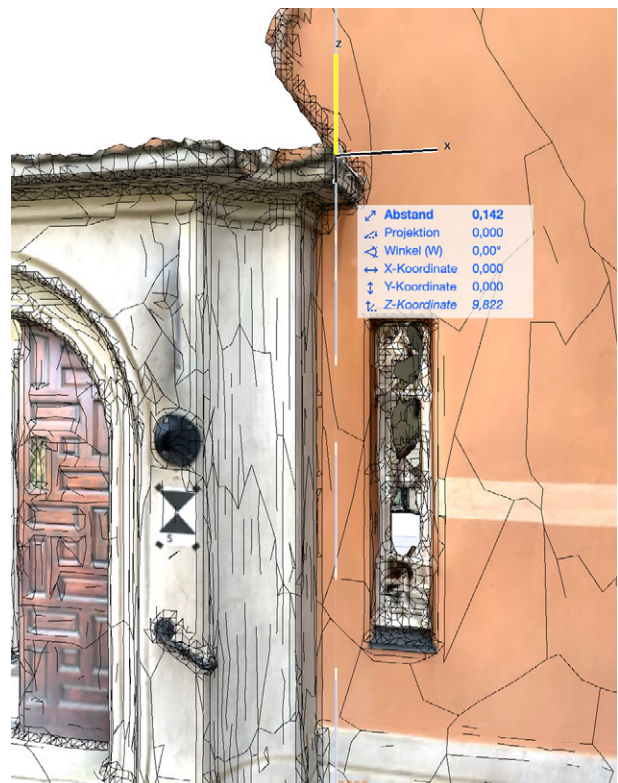
Fig. 2.6.44: Screenshot Archicad, measuring the entrance facade
