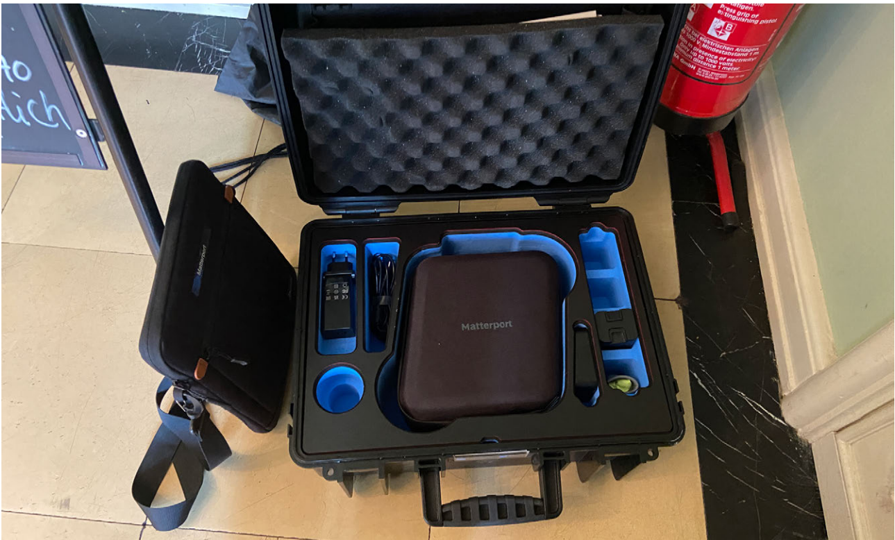
Fig. 2.2.9: Matterport Pro 3 Performance Kit
