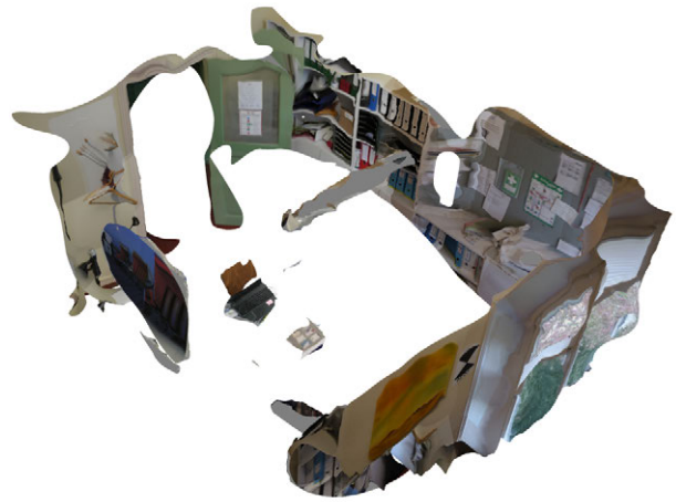
Fig. 2.4.10: Mesh and Texture with Autodesk Recap of the Office Room
