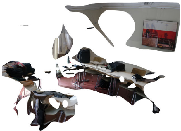
Fig. 2.4.11: Mesh and Texture with Autodesk Recap of the Office Room
