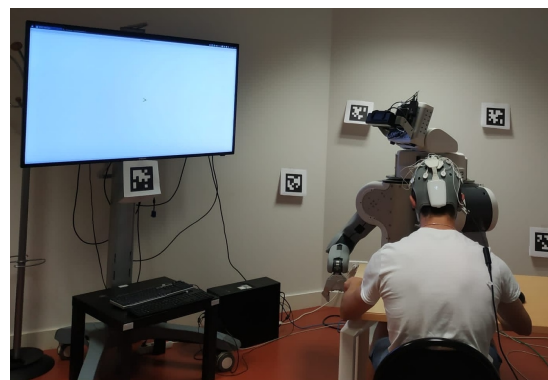
Figure 1: A typical HRI experimental setup, with a participant equipped with electrophysiological measurement devices sat in front of a PR2 robot.
