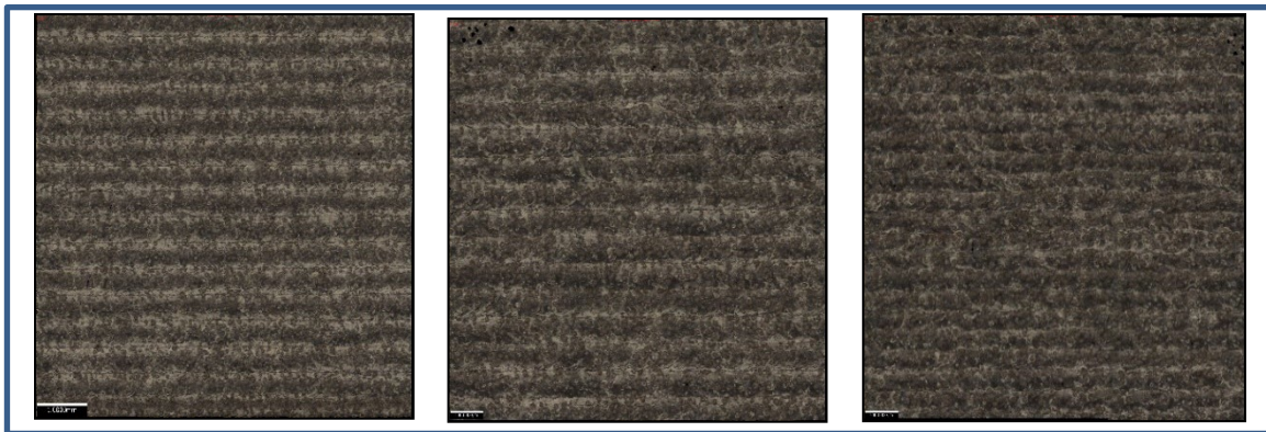
Fig. 2: A visual representation of how the deposition pattern evolves with varying bead overlap, from 10% to 30% to 50%
