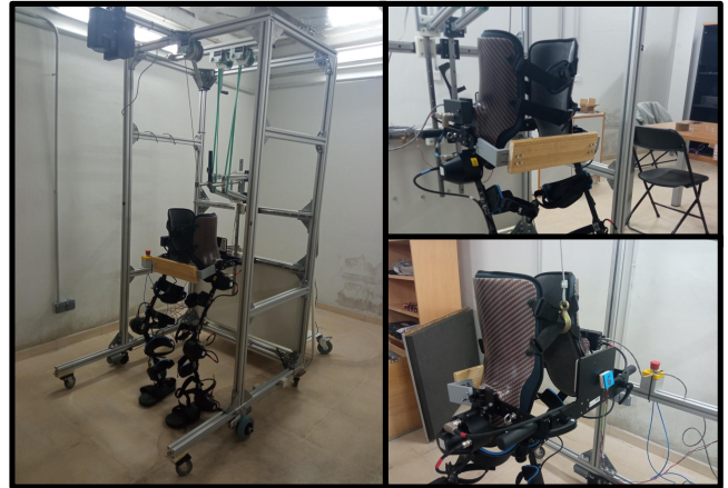
FIGURE 4: Experimental setup for the H3 exoskeleton.
