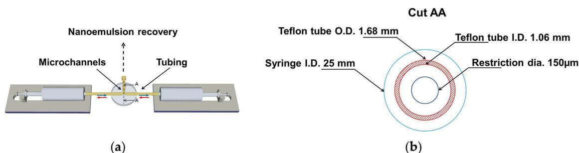
**Figure 1.** Schematic drawing of the microprocess to prepare the polymerizable nanoemulsion (not at scale, (a)), dimensions of the different channels in cut AA (b).
