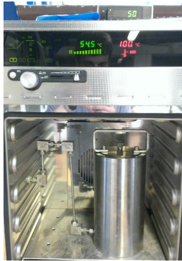
Figure 2: Pressure vessel in oven regulated at 60°C
