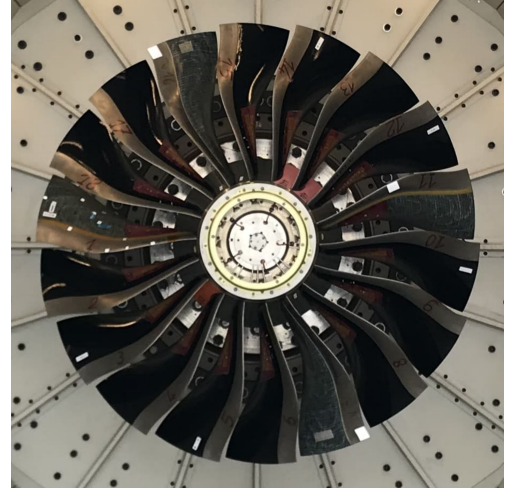
Fig. 7: Blade and fan instrumentation.
