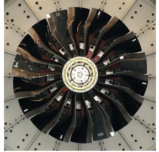
Fig. 7: Blade and fan instrumentation.
