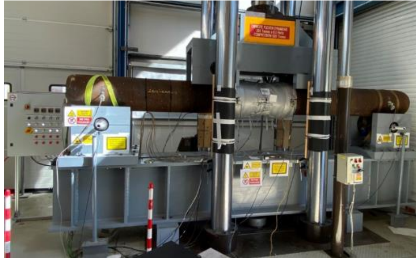
Figure 6: Test pipe and four points bending loading device
