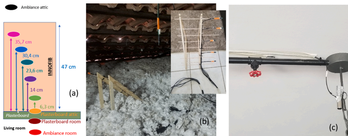
Fig. 3. (a) Sensor position, (b) wooden scale supporting the T and RH sensors, (c) sensor inside the room.
