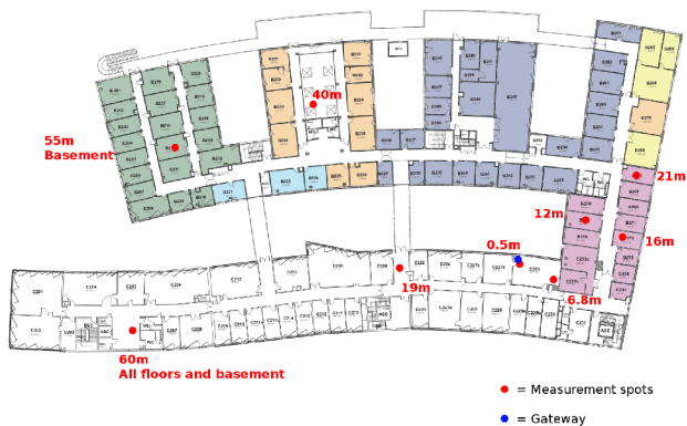
Figure 3. Gateway location and measurement spots in the building
