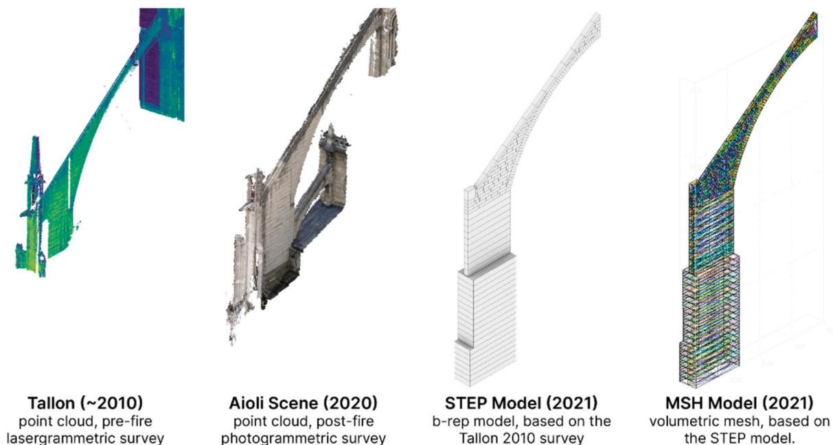
Fig. 7. Four geometric representations of the T17 flying buttress: pre-fire lidar and post-fire photogrammetry surveys, STEP and MSH models for supporting mechanical simulation. Each geometry is stored in the Data Lake and linked in the Knowledge Graph.
