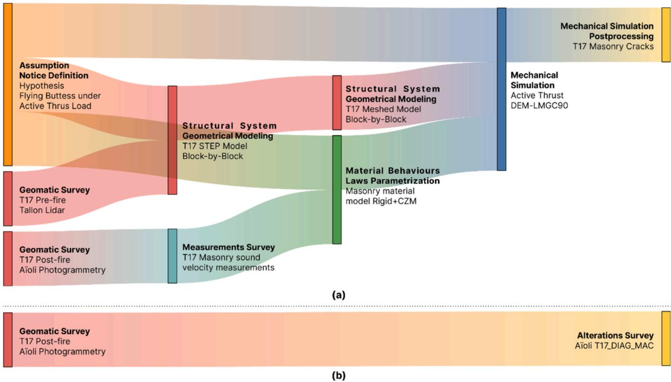
Fig. 10. Provenance visualization for two *Builtwork Feature* instances related to the T17 Flying Buttress: (a) a crack predicted by the *Active Thrust* simulation scenario and (b) a crack observed during the visual inspection of alterations.
