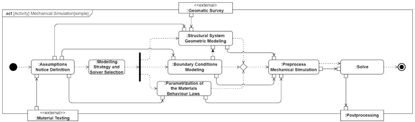
Fig. 3. SysML Activity diagram outlining the tasks and information flows tied to numerical simulation preparation, modeling, and computing.
