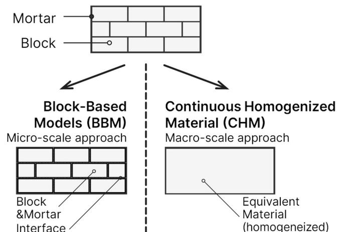
Fig. 2. Block-Based Models (BBM) and Continuous Homogenized Material (CHM), two strategies for modeling masonry-based structures.
