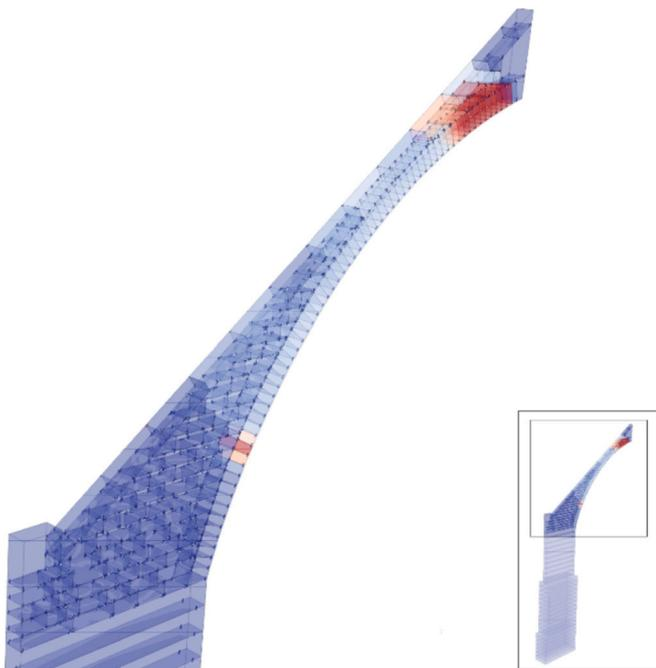
Fig. 9. Mechanical simulation prediction for a choir flying buttress under active thrust load. The DEM-based LMGC90 solver outlines block panel rotation and the apparition of a crack at the head of the flying buttress.
