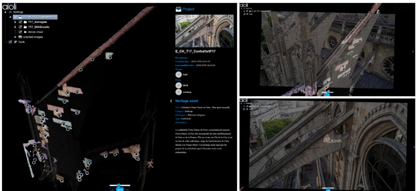
**Fig. 8.** Visual survey masonry information recorded on the Aioli platform, with annotations applied to both the photogrammetric point cloud (left) and corresponding photos (right).
