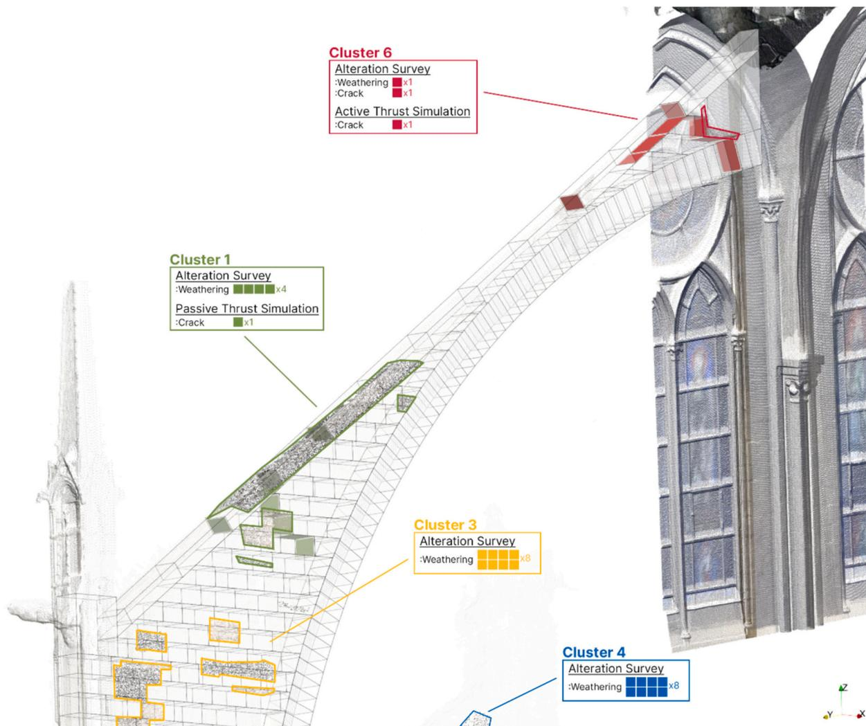
Fig. 12. Spatial clustering results of *Builtwork Features* instances, corresponding to observed or predicted alteration during the structural diagnosis of the T17 flying buttress. Each instance is represented as a square and classified according to its type from the ICOMOS glossary for stone alteration [63].
